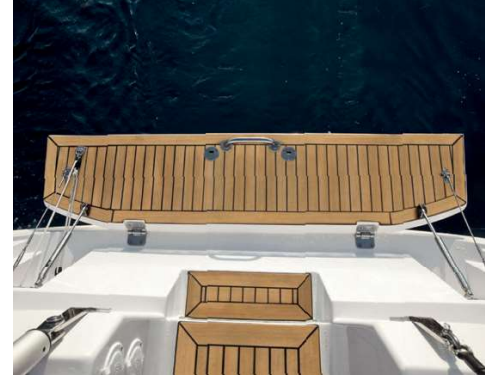
The drop-down bathing platform offers easy access to the sea, while increasing the surface area on deck.
