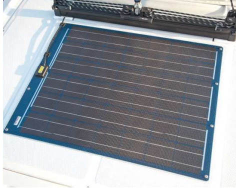
A solar panel can be mounted on the cabin roof in order to ensure enough power even on longer cruising hauls. Available as an option.
