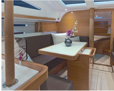
Double size saloon table that folds down and creates additional berth in the saloon.
